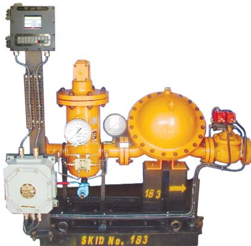
MSA meter skid with Toptech SMP controller
