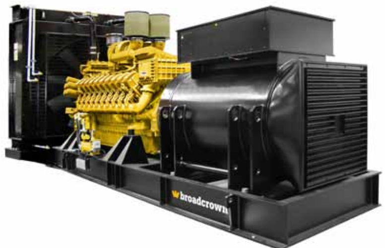
BCMU 2800P-50: engine 20V 4000 G63 (FO), alternator LVSI 804 S2
